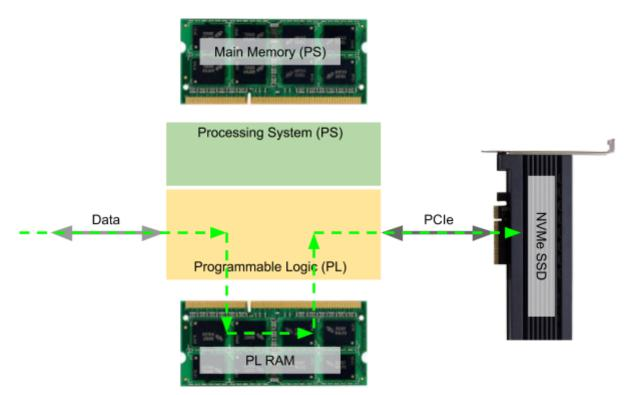
Data flows between PL (for example entering the FPGA via GTX or GTH or GTY Multi-Gigabit Transceivers) and the PCIe direct-attached NVMe SSD, with an buffer in between using PL-attached DDR4 RAM (please refer to the FAQ section of our products page [http://MLEcorp.com/nvme] for details regarding this buffer).
