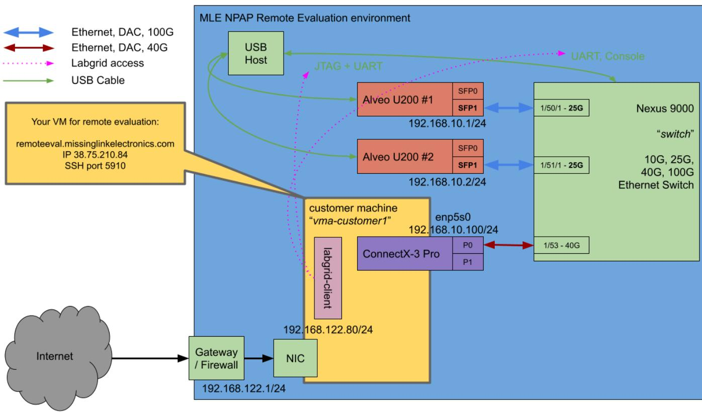
Once you have been granted access to the MLE NPAP Remote Evaluation environment, you will be in charge of what is called “Customer Machine” in the diagram above. This machine is a fully virtualized machine with access to the following components:
